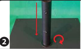
Thread the Shaft onto the Base Plate Threaded Bolt. As the Shaft tightens against the Base Plate, be sure the Shaft ends snuggly against the Base Plate. Do not over tighten, this may damage the enameling on the Washer.
