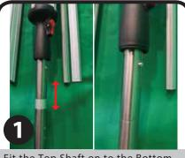
Fit the Top Shaft on to the Bottom Shaft. Slide the two halves together and verify proper connection by observing snap-lock has engaged.
