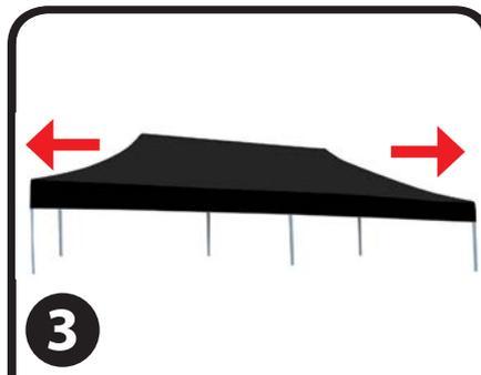
Expand frame out fully by having each person move to the middle leg of the 20' side. Grasp at bottom of the v. Lift up and step backwards at the same time until tent is fully opened.
